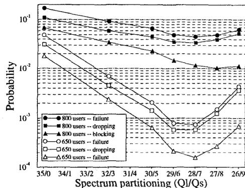
Figure 9: Moving users: loss probabilities vs spectrum partitioning.
