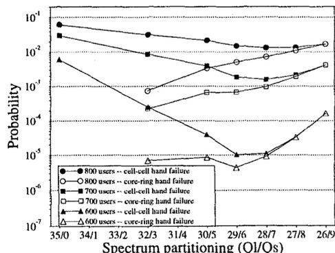
Figure 10: Moving users: handover failure probabilities vs spectrum partitioning.
