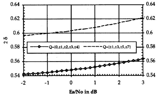
Fig. 3. Threshold value as a function of  $E_s/N_o$  and metric set.
