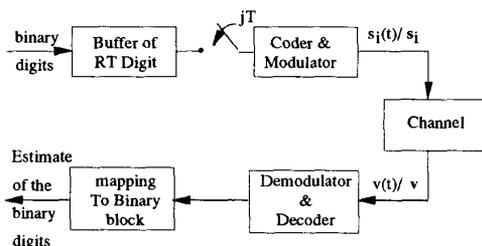
Fig. 1. A general block coded digital data communications system.
