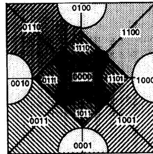
Fig. 5. Schematic description of the signal space partition for QPSK,  $Q=2$ .
