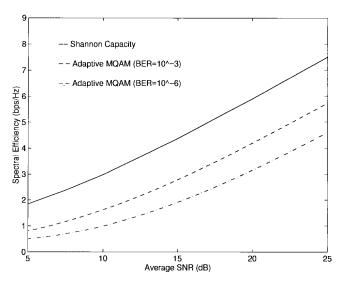
Fig. 3. Efficiency in Rayleigh fading.
