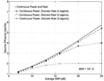
Fig. 5. Discrete-rate efficiency in Rayleigh fading.
