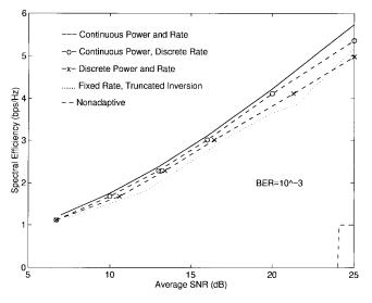
Fig. 9. Efficiency in Rayleigh fading.
