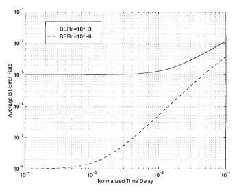
Fig. 11. Effect of normalized delay  $(\tau f_D)$  on BER.
