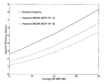
Fig. 2. Efficiency in lognormal shadowing ( $\sigma = 8$  dB).
