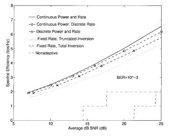
Fig. 8. Efficiency in lognormal shadowing ( $\sigma = 8$  dB).
