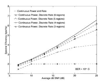
Fig. 4. Discrete-rate efficiency in lognormal shadowing ( $\sigma = 8$  dB.).
