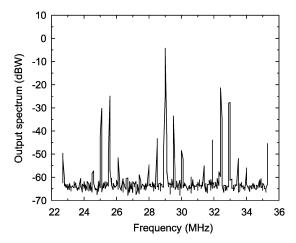
Fig. 11. Expanded view of the experimental output power spectrum about the input-drive frequency.  $V_{DD}=72~\mathrm{V}$  and  $P_{\mathrm{in}}=5.15~\mathrm{W}$ . It shows the coexistence of two oscillation frequencies at approximately 4 MHz and 500 kHz. This is in agreement with the envelope-transient simulation of Fig. 10.
