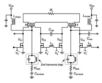
Fig. 13. Amplifier schematic with stabilization network. The stabilization network consists of a stabilization resistor  $R_{\rm stab}$ , a second harmonic trap, and a dc-blocking capacitor  $C_{\rm dc-block}$ .
