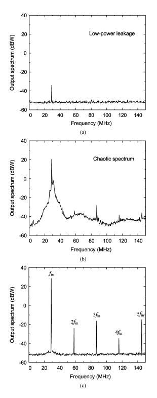
Fig. 3. Variation of the measured output power spectrum when increasing the input power. (a)  $P_{\rm in}=4$  W, showing leakage power at the input-drive frequency. (b)  $P_{\rm in}=10$  W, showing a chaotic spectrum. (c)  $P_{\rm in}=16.5$  W, showing the proper spectrum in switching-mode operation.
