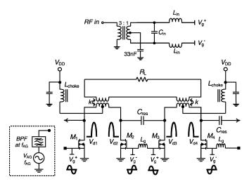
Fig. 1. Schematic of the class-E/ $F_{\rm odd}$  PA with sketches of the voltage waveforms at the main circuit nodes. Two push-pull pairs are formed by  $M_1-M_2$  and  $M_3-M_4$ , although the transistors in each pair are in different transistor packages. The AG with an ideal bandpass filter inside the dashed box is not a part of the amplifier, but will be connected to one of the drain terminals for the stability analysis in Section V.
