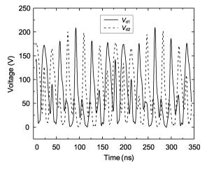
Fig. 7. Comparison of two simulated drain voltage waveforms  $V_{d1}$  and  $V_{d2}$  in the same push–pull pair. The slowly varying envelopes at the oscillation frequency appear to be in-phase, whereas the fast-varying carriers are out-of-phase.
