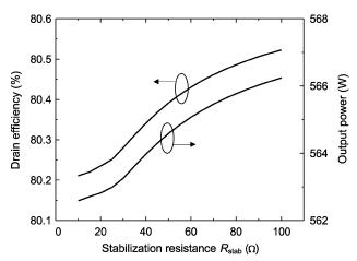
Fig. 16. Variation of the amplifier drain efficiency and output power versus the value of the stabilization resistance. The drain bias voltage is assumed as  $V_{DD}\,=\,72\,$  V.
