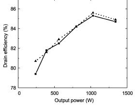
Fig. 17. Measured drain efficiency versus the output power. Solid line: stabilized PA. Dashed line: original PA. Compared to the original PA, the drain efficiency is degraded by less than 0.4% for all output power levels, except for 240 W, which shows 1.3% degradation.
