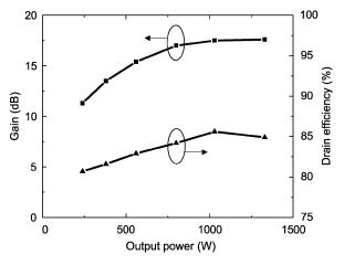
Fig. 2. Variation of the gain and drain efficiency of the class- $E/F_{\rm odd}$  PA versus the saturated output power. The output power is varied by changing the drain bias voltage.
