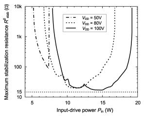
Fig. 15. Variation of the maximum value of stabilization resistance  $R_{\rm stab}^0$  versus the input-drive power  $P_{\rm in}$  obtained through bifurcation analysis. Three different drain bias voltages have been considered.
