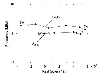
Fig. 5. Evolution of the critical poles with increasing input power for  $V_{DD}=72~\rm{V}$ . For simplicity, only poles in the upper half of the complex plane have been represented. The input power has been increased from 5 to 15 W by 1-W step. The poles cross to the right-hand side of the complex plane for  $P_{\rm in\_Hl}=6.1~\rm{W}$  and return to the left-hand side for  $P_{\rm in\_Hu}=13.5~\rm{W}$ .
