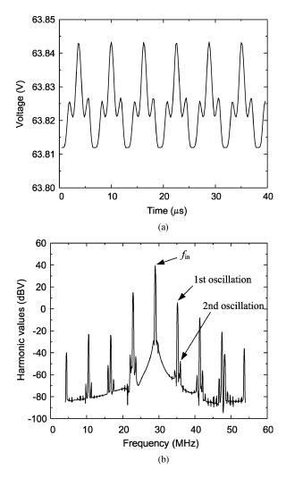
Fig. 10. Envelope-transient simulation of the amplifier. (a) Time-domain evolution of the magnitude of the  $f_{\rm in}$  harmonic component of the drain voltage when a two-fundamental basis at  $f_{\rm in}$  and  $f_a$  is considered. (b) Spectrum of the harmonic component showing the presence of two oscillation frequencies.
