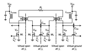
Fig. 8. Schematic of the push–pull amplifier showing the virtual-ground and virtual-open planes at the oscillation frequency.
